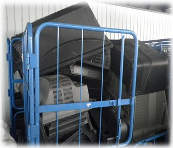
CRT TV casing: ~ 120,000 mg/kg of PBDE
