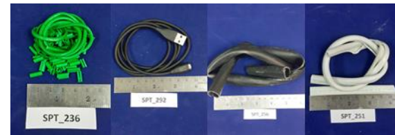
PVC sheaths from wires and cables (n=56)
