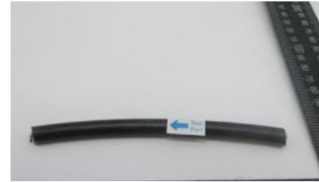
Electical cable with PVC sheathing
